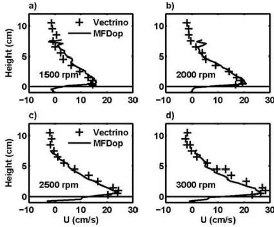
**Figure 7:** Comparison between mean velocity profiles measured using a Nortek Vectrino ADV (values indicated with a +), and multi-frequency Doppler (indicated by a solid line). Profiles a, b, c, and d correspond to increasing flow speeds as regulated by pump speeds of 1500, 2000, 2500, and 3000 rpm respectively.
