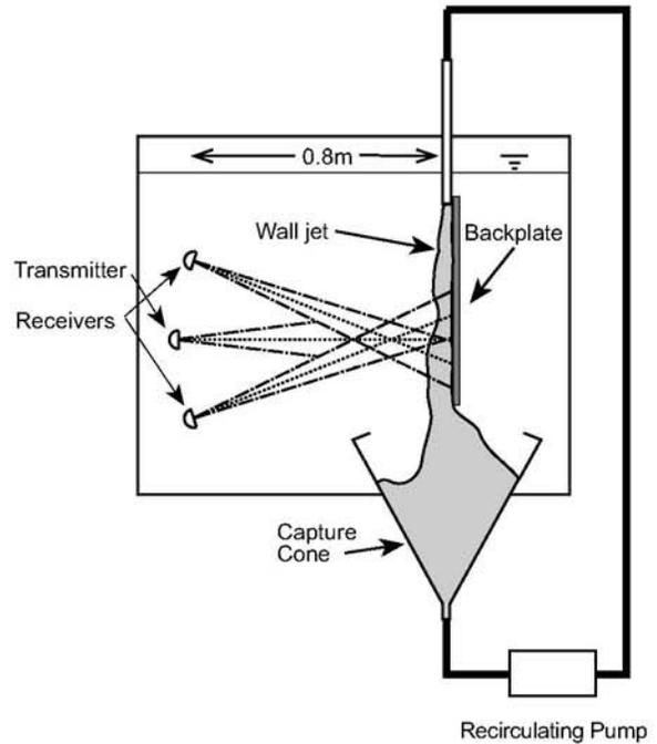
**Figure 5:** Wall jet experiment configuration. A sediment laden water jet is directed vertically into a  $1 \text{ m}^3$  tank parallel to the edge of a backplate. The Doppler profiler is configured to sample a profile across the jet.
