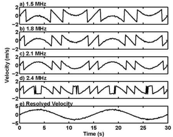
**Figure 4:** Example of velocities recovered from simulated backscatter plus noise at a) 1.5 MHz, b) 1.8 MHz, c) 2.1 MHz, d) 2.4 MHz. For these discrete frequency velocity estimates, output velocities are restricted by the ambiguity velocity. e) shows the reconstructed velocity using the multi-frequency information.
