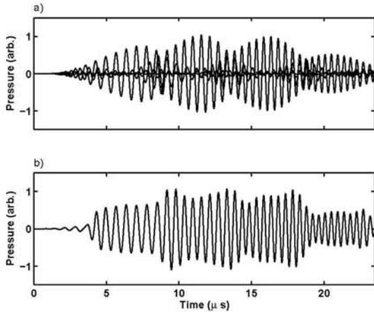
**Figure 2:** Transmit pulse template. a) Constituent pulses at 1.5, 1.8, 2.1, and 2.4 MHz and b) formed multi-frequency pulse. Each constituent is  $4.7 \mu\text{s}$  in duration, the transducer has a center frequency of 1.8 MHz and bandwidth of 800 kHz.
