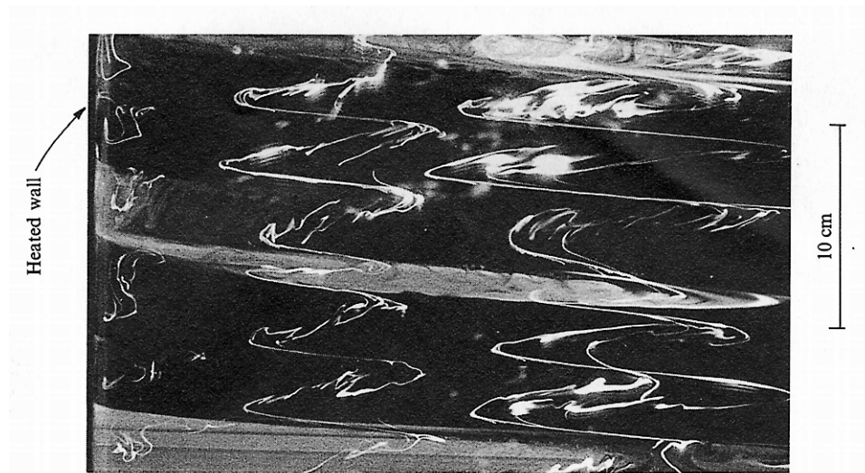
Figure 3. (Reproduced by permission of Cambridge University Press, from Tanny and Tsinober, 1988, figure 17.) The heated sidewall experiment at a later stage, using fluorescent dye traces to show the stable shear flow at the interfaces (nearly horizontal straight lines) and the unstable shear flow within the layers (inclined convoluted lines).
